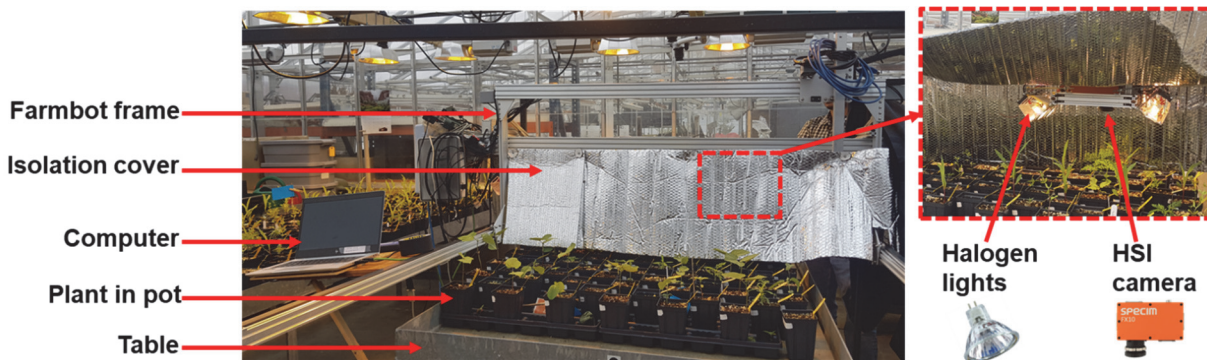
Figure 2. Demonstrations of HSI system used for soybean and weeds in greenhouse environment.
